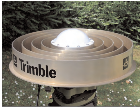
Abb. 11a: Trimble-Choke-Ring-Antenne (TRM29659.00) ohne Radom (Foto: Galitzki)
